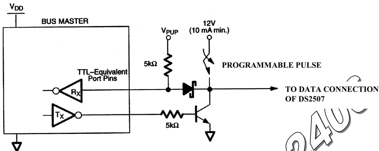
The diode and Programming Pulse circuit are not required if one does not intend to program the EPROM cells.
