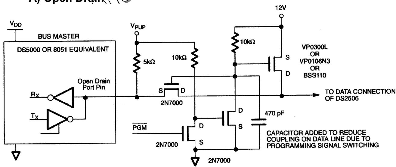
The interface is reduced to the 5 k $\Omega$  pullup resistor if one does not intend to program the EPROM cells.
