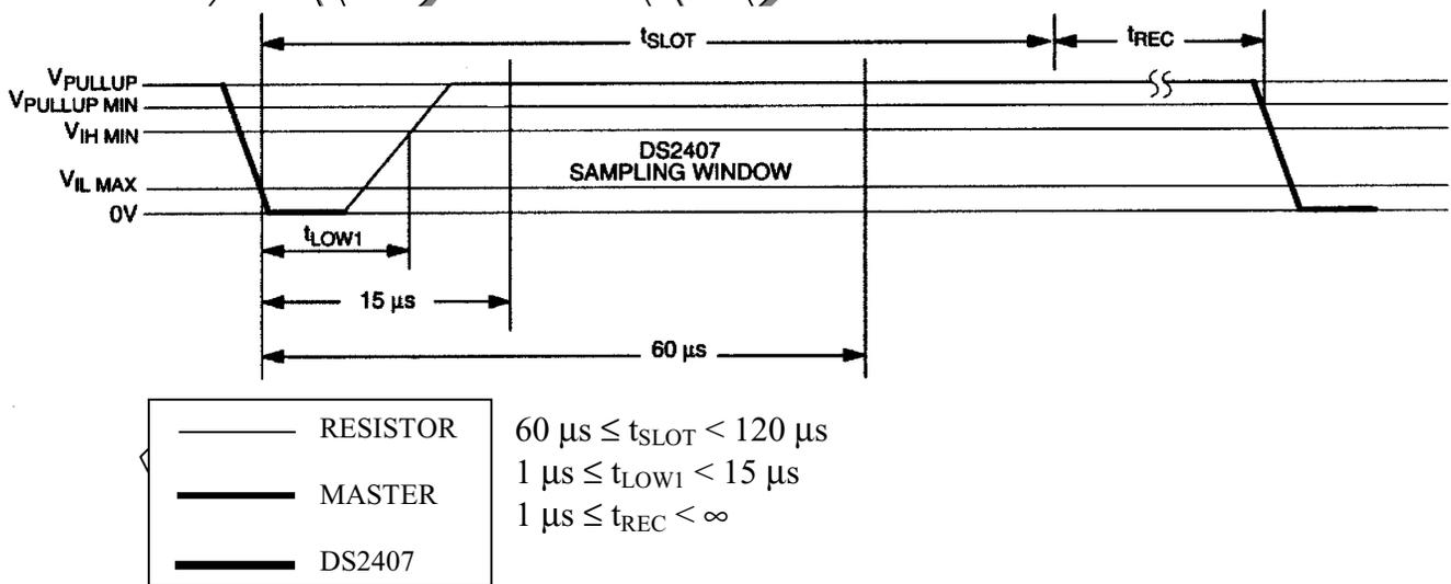
**READ/WRITE TIMING DIAGRAM Figure 15 (cont'd)****Write-0 Time Slot**
