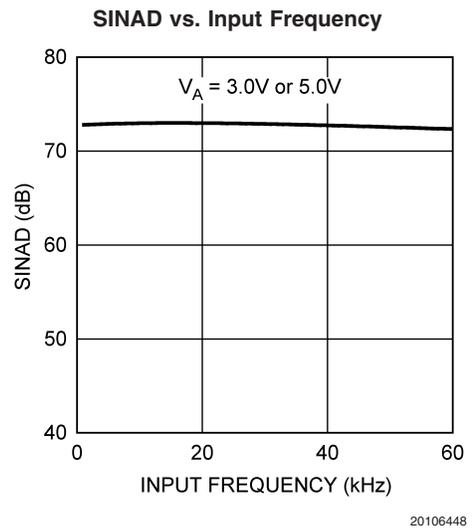
**Typical Performance Characteristics**  $T_A = +25^\circ\text{C}$ ,  $f_{\text{SAMPLE}} = 200 \text{ kSPS to } 500 \text{ kSPS}$ ,  $f_{\text{SCLK}} = 3.2 \text{ MHz to } 8 \text{ MHz}$ ,  $f_{\text{IN}} = 40.2 \text{ kHz}$  unless otherwise stated. (Continued)
