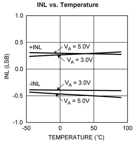
**Typical Performance Characteristics**  $T_A = +25^\circ\text{C}$ ,  $f_{\text{SAMPLE}} = 200 \text{ kSPS to } 500 \text{ kSPS}$ ,  $f_{\text{SCLK}} = 3.2 \text{ MHz to } 8 \text{ MHz}$ ,  $f_{\text{IN}} = 40.2 \text{ kHz}$  unless otherwise stated. (Continued)
