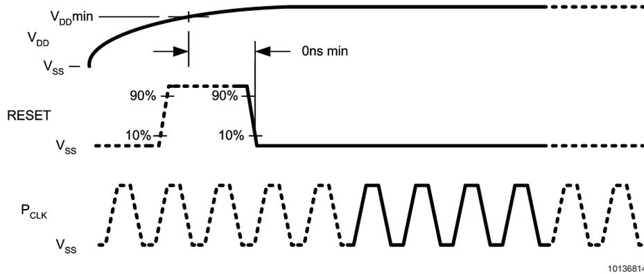
FIGURE 5. Power-On Reset Sequence with Manual Reset
