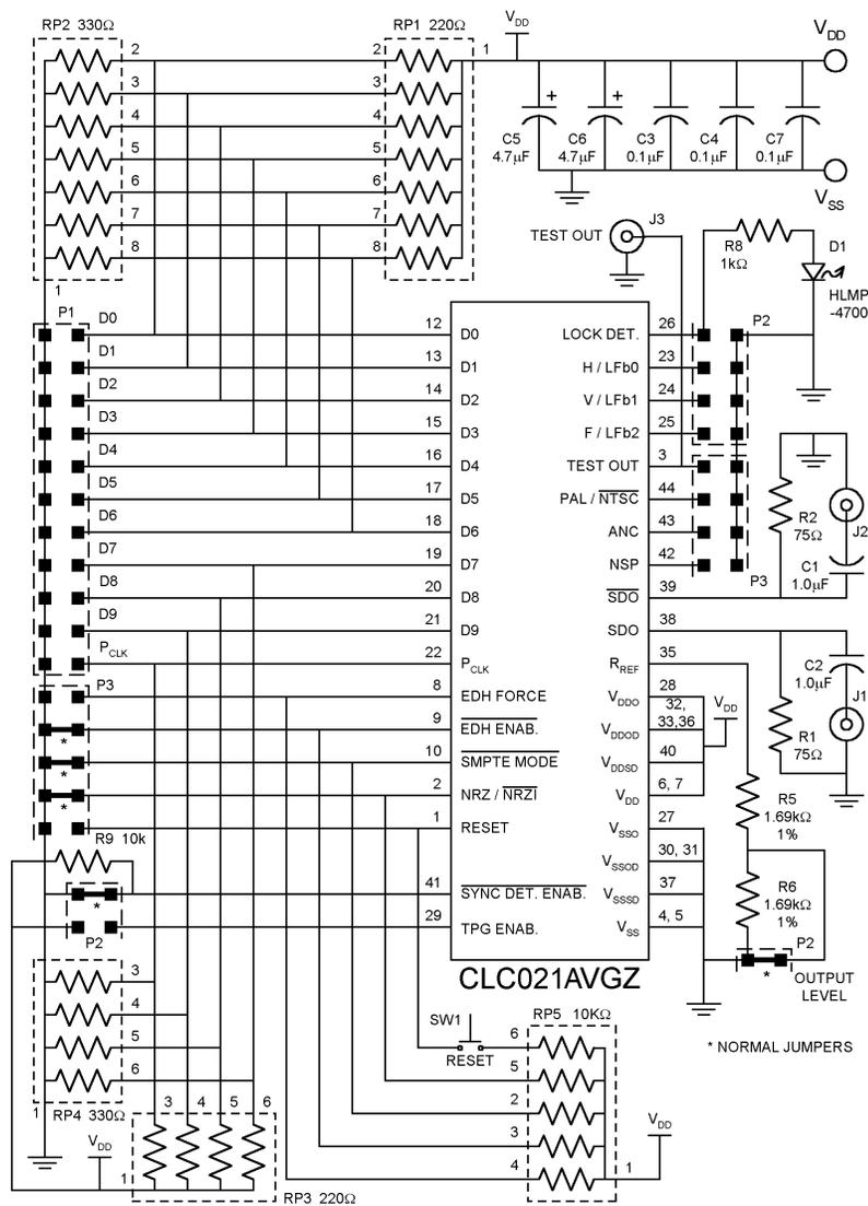
Connect LOCK DETECT to TPG ENABLE for test pattern generator function.
