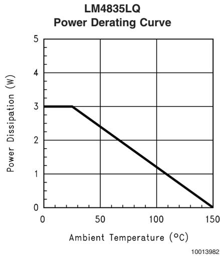
**Note 19:** These curves show the thermal dissipation ability of the LM4835MTE at different ambient temperatures given these conditions:
