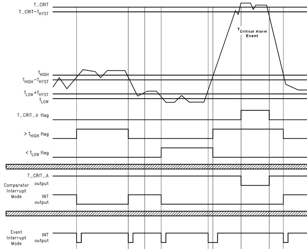
**Note:** Event Interrupt mode is drawn as if the user is reading the part. If the user doesn't read, the outputs would go low and stay that way until the LM76 is read. 10101506
